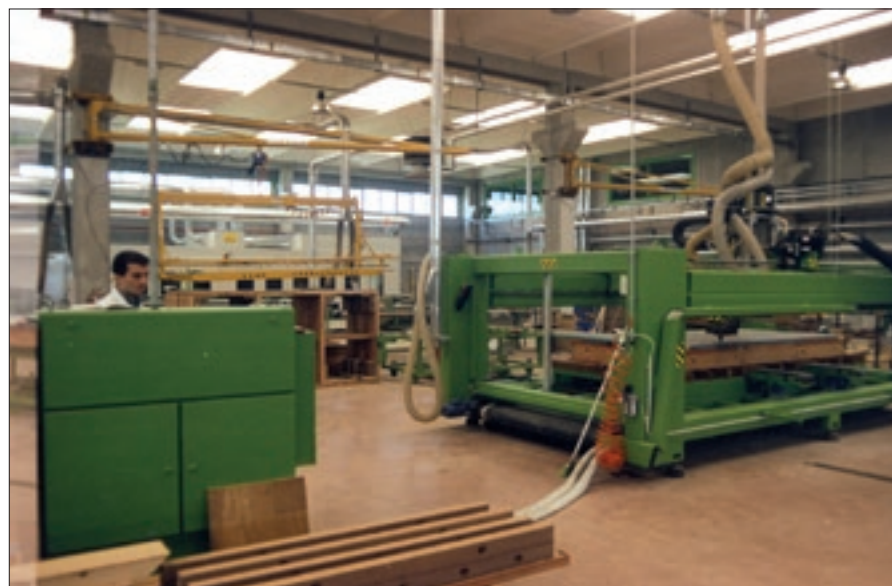
Machine for rectification and squaring of billiard table
